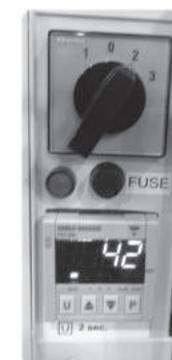
This heater is fitted with a voltage protection device. If the supply voltage is higher or lower than required, the machine will shut down and the red warning light will illuminate.
